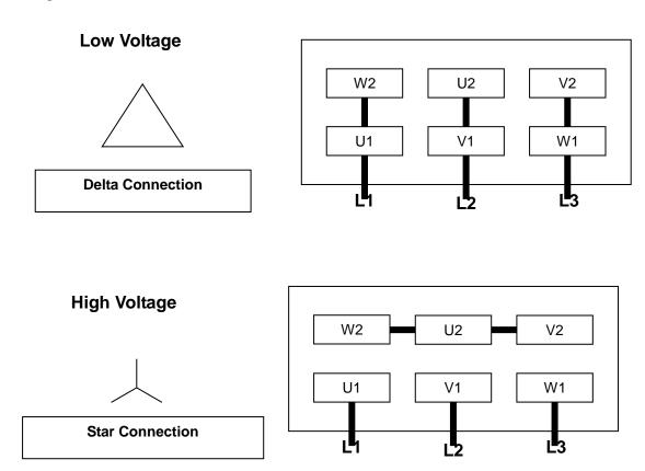
The motor must be connected according to the electrical codes through a fused switch in order to protect the motor against electrical or mechanical overload conditions. The overload of the motor starter must be set at a level equal to the full load motor current listed on the motor nameplate.
